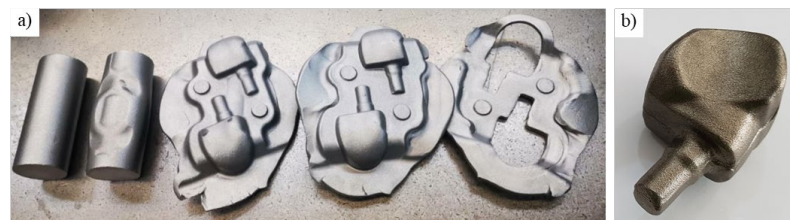
a) The workpiece after forming each operation step, and b) The workpiece after forming by the hot forging process
