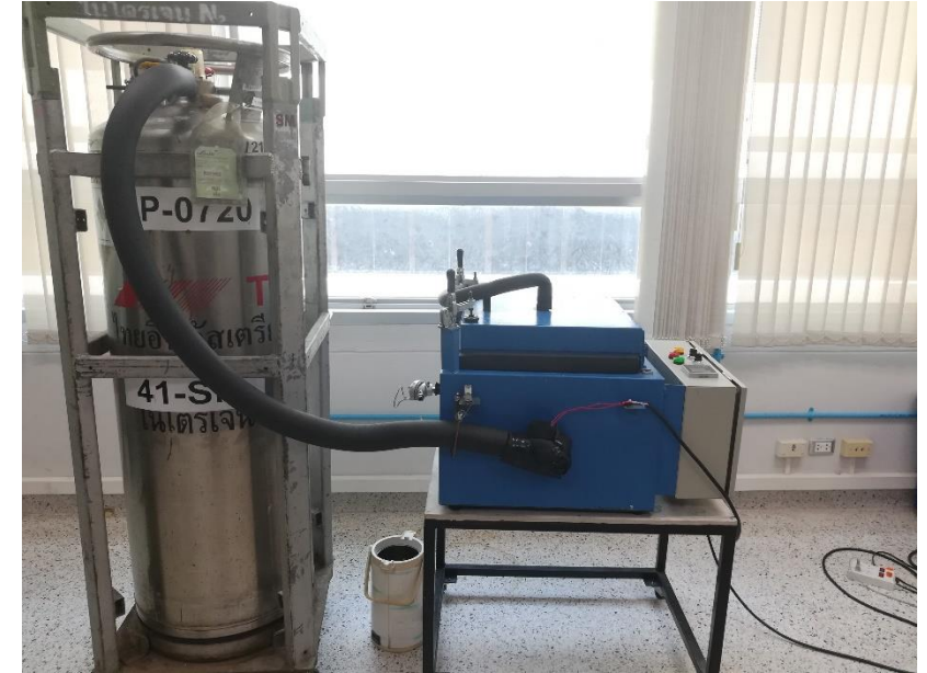
Cryogenic treatment , Chovachot, Min. Temperature -140 °C Max. during time 4 hours
